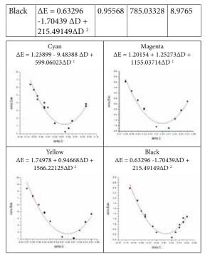
**Fig. 3** Graph showing the scatter plot and fitted lines for uncoated paper
