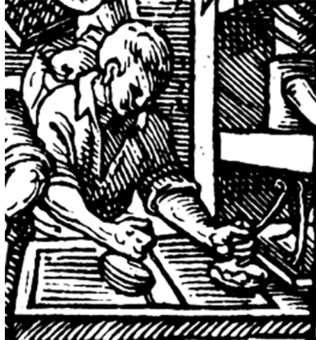
Figure 7. Manual application of ink using the tampon and exposing the prints 18
