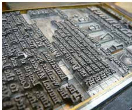
Figure 5. Composite printed form of individual characters of lead alloy 16
