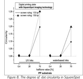
Figure 8. The degree of dot circularity in SquareSpot samplea printed on polypropylene
