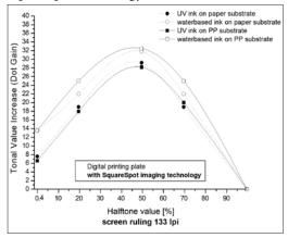
Figure 11. Dot gain curves of SquareSpot samples with 133 lpi
