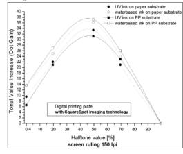
Figure 12. Dot gain curves of SquareSpot samples with 150 lpi
