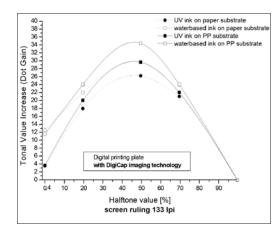
Figure 9. Dot gain curves of DigiCap samples with 133 Ipi
