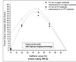
Figure 10. Dot gain curves of DigiCap samples with 150 lpi
