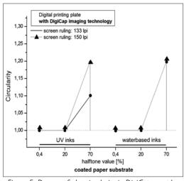
Figure 5. Degree of dot circularity in DigiCap samples printed on paper
