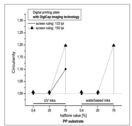
Figure 6. Degree of dot circularity in DigiCap samples printed on polypropylene
