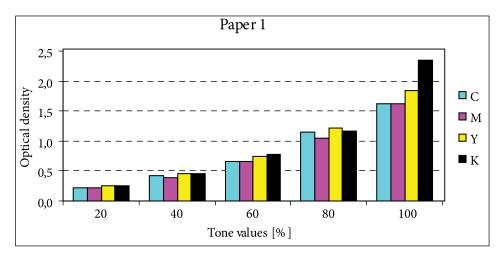
Figure 1: Optical density of CMYK prints at Paper 1.
