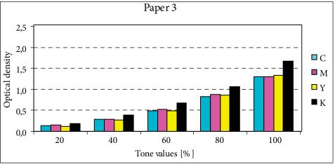
Figure 3: Optical density of смүк prints at Paper 3.
