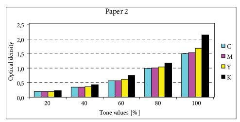
Figure 2: Optical density of CMYK prints at Paper 2.
