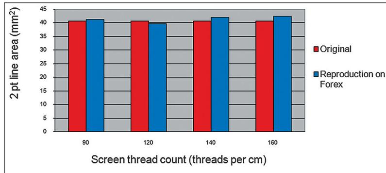
Figure 2. Areas of 2 pt thick lines printed on Forex with different thread counts
