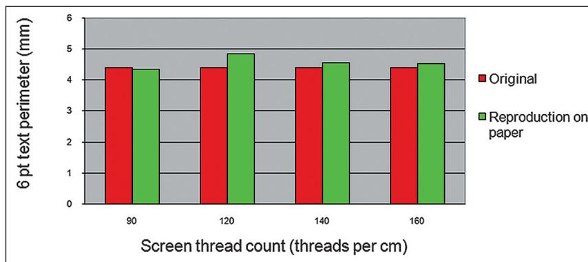
Figure 10. Perimeter of 6 pt letter e printed on paper with different thread counts
