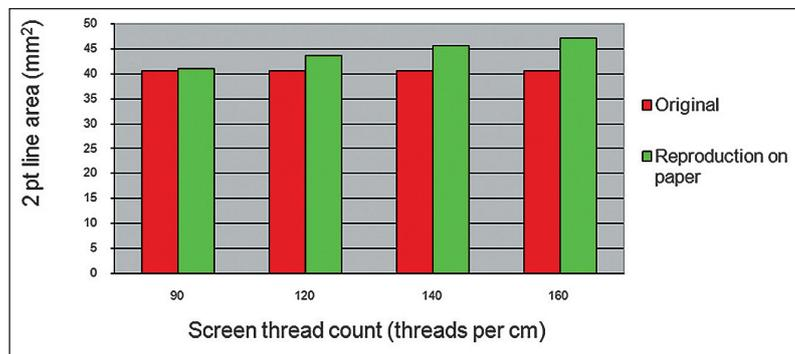
Figure 4. Areas of 2 pt thick lines printed on paper with different thread counts
