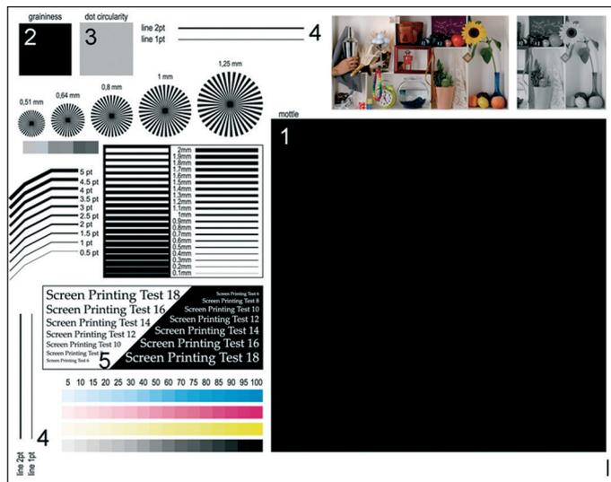
Figure 1. Test image used to evaluate reproduction of image elements (1 – area for macro non-uniformity control, 2 – area for micro non-uniformity control, 3 – element for dot circularity control, 4 – lines of 1 and 2 point width, 5 – text in positive and negative ranging from 6-18 pt)
