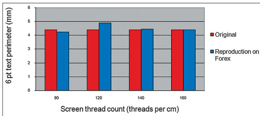
Figure 9. Perimeter of 6 pt letter e printed on Forex with different thread counts
