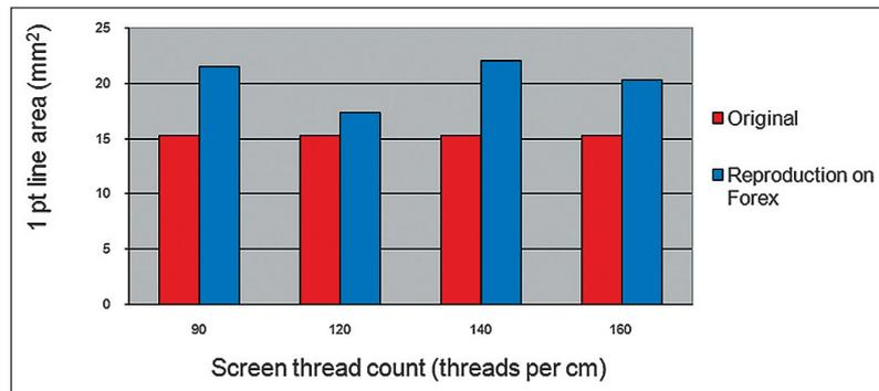
Figure 3. Areas of 1 pt thick lines printed on Forex with different thread counts
