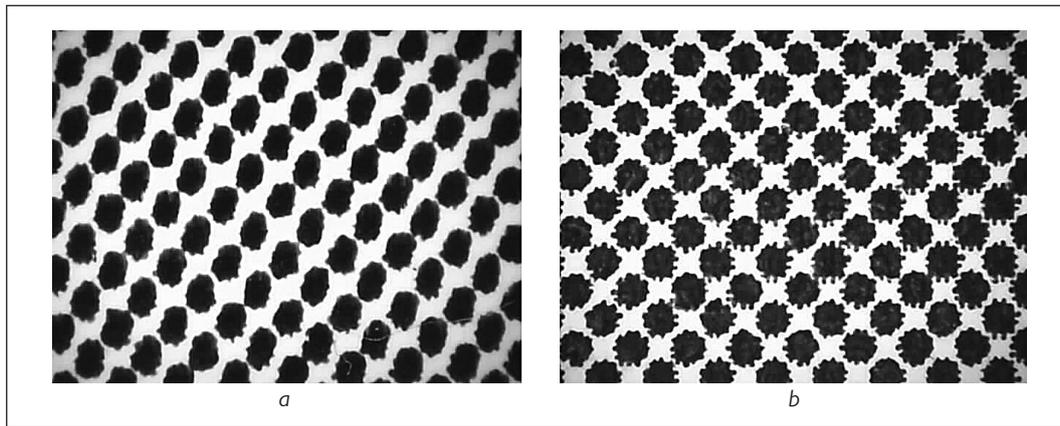
Figure 11. Dot structure of 30% TV detected with Sibress Pit camera. Substrate: a – Forex, b – paper
