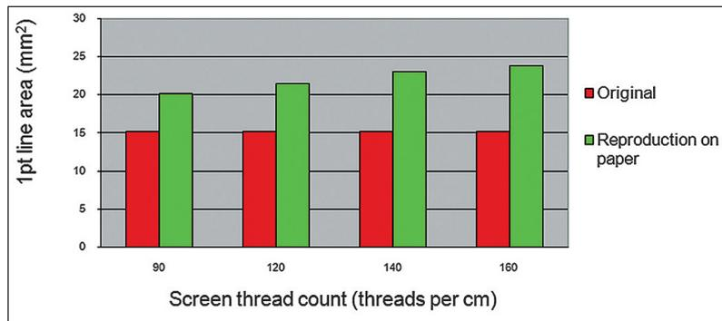
Figure 5. Areas of 1 pt thick lines printed on paper with different thread counts
