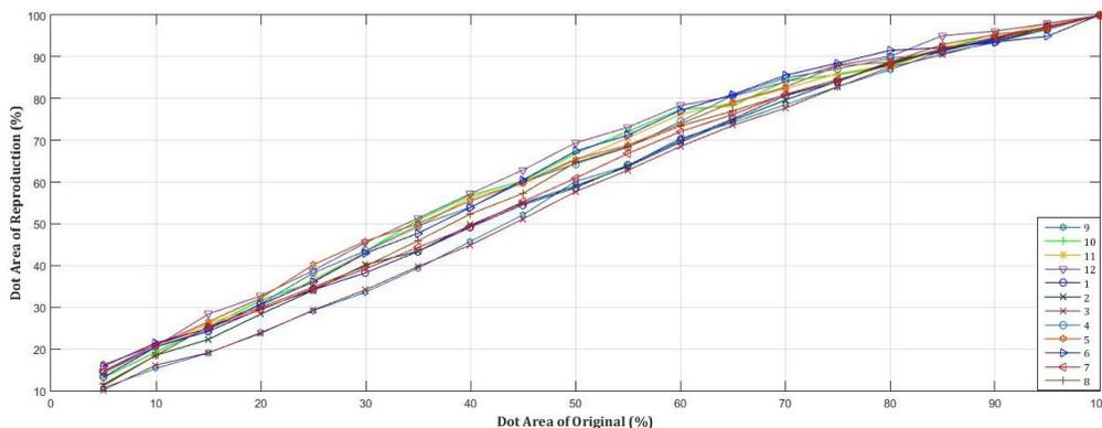
*Figure 4 Tonal Reproduction Curve for Dot Area*
