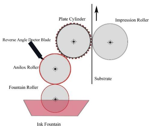
**Figure 1** Schematic diagram of flexographic printing unit: the well metered ink from the surface of anilox roller is transferring on to the flexographic plate and then to the substrate.
