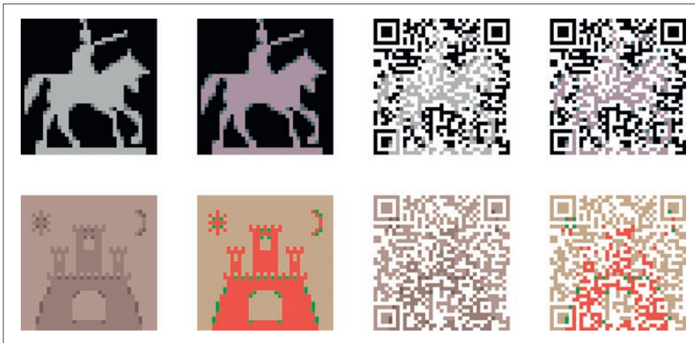
Figure 1. Color data modules in the QR code and their values in greyscale.
