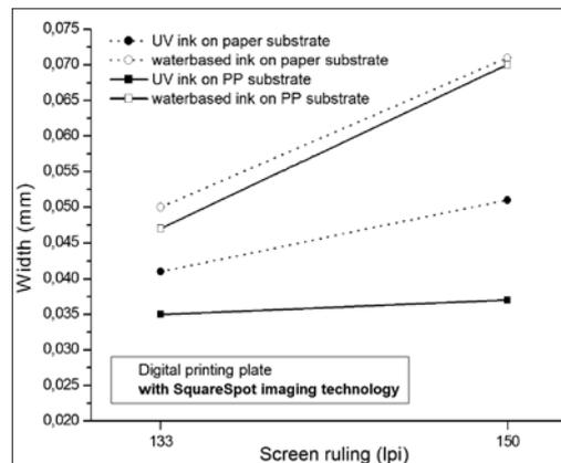
Figure 2. Line width of SquareSpot samples
