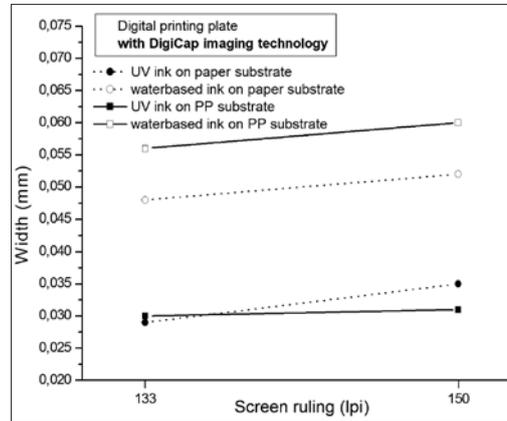
Figure 1. Line width of DigiCap samples
