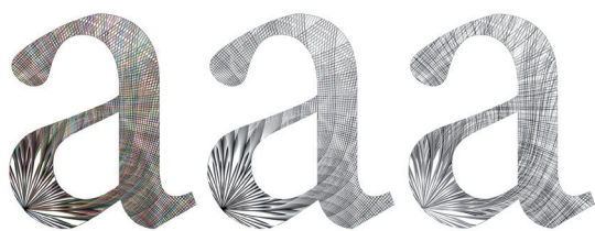
Figure 4. Letter mask on rosette with C, M, and Y random coverage values, with gradient rise in K coverage values. Left: CMYK, right: black channel response simulation in the NIR part of the spectrum
