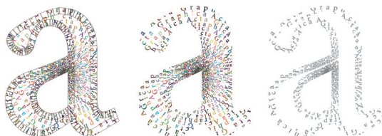
Figure 5. Letter mask on rosette with C, M, Y, and K random coverage values. Left CMYK, right: response simulation of the black channel in the NIR part of the spectrum
